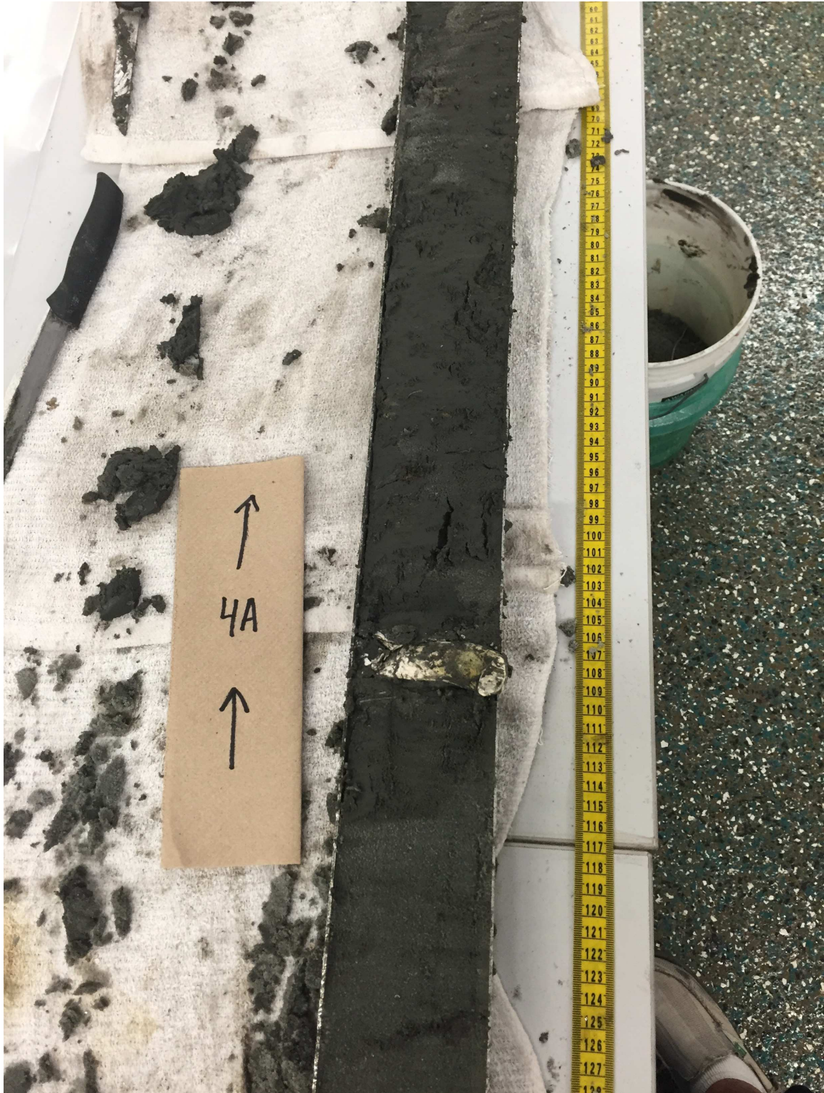
Figure 19: Sediment core of the paleommarsh from Vibracore 4. Note the black color, oyster shell, and root fragments.
