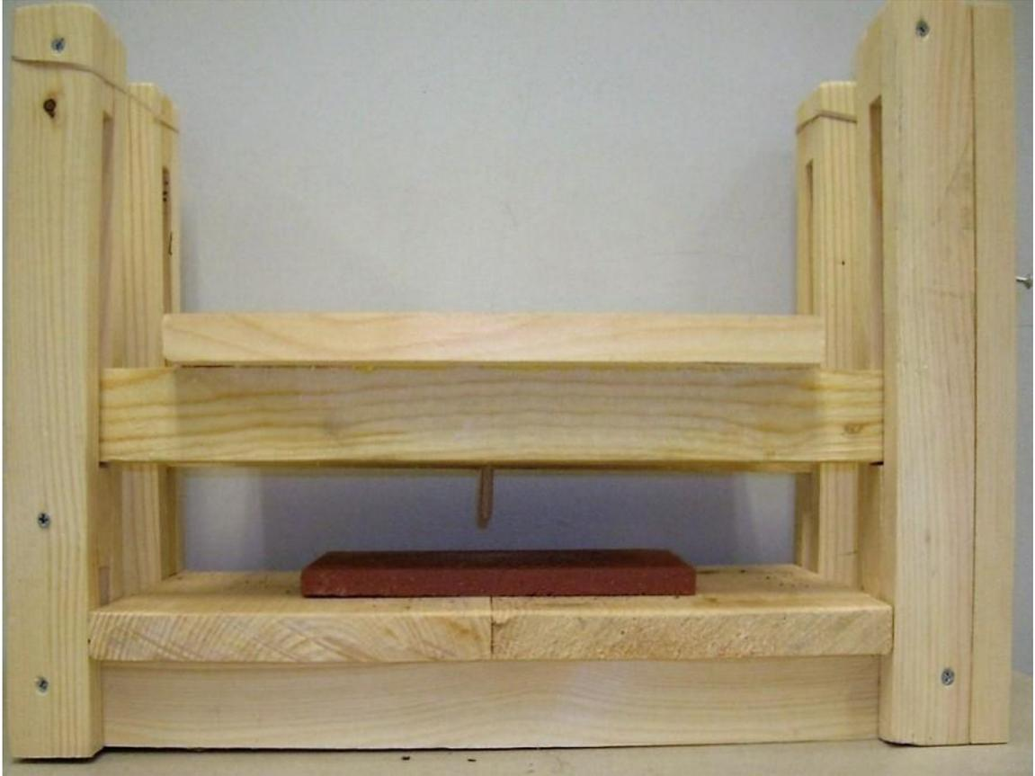
**Figure 2:** The hand-made device designed to measure the compression strength of shells.
