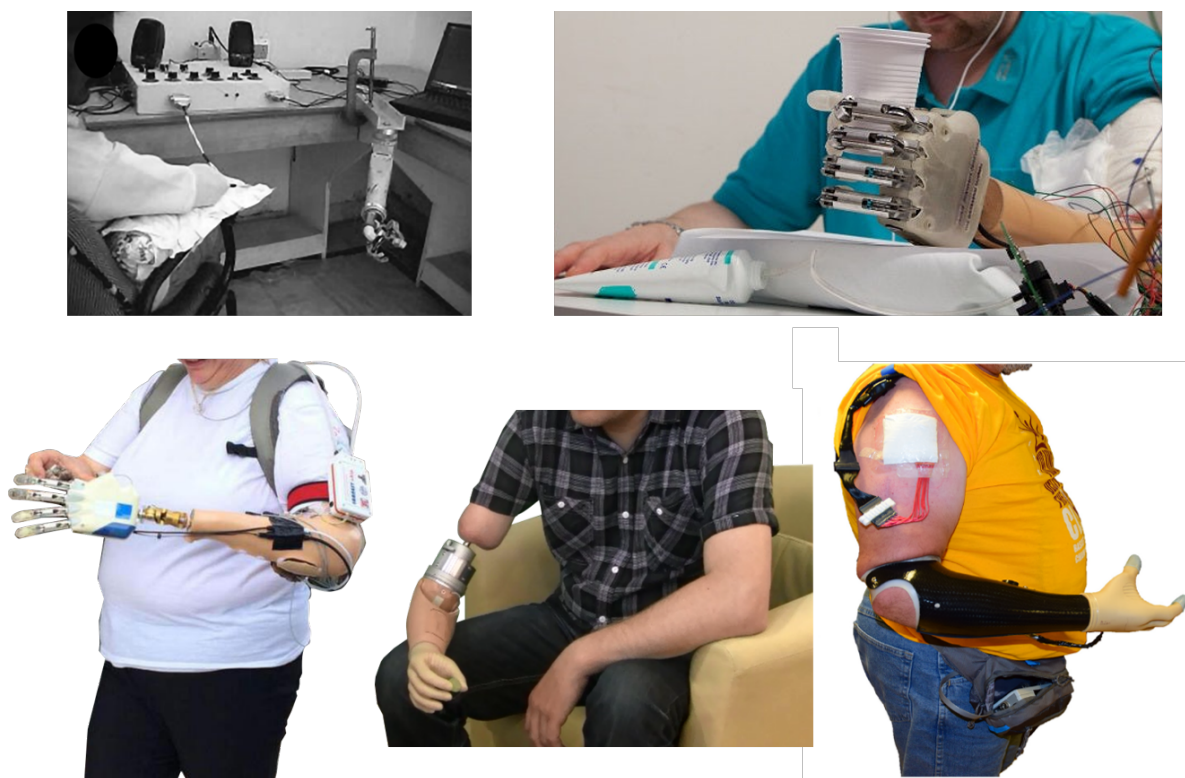
Figure 7.2: Neural stimulation for closed-loop prosthetic control: a changing trend from experiments confined within controlled environments (top) to amputees' daily environments and more realistic use scenarios (bottom). Top-Left) Experiments from Dhillon and Horch showed that tactile as well as proprioceptive sensations could be elicited using intraneural electrodes [63]. Top-Right) Experiment of object compliance recognition performed within the framework of the E.U. funded NEBIAS project, efforts that ultimately allowed a transradial amputee to walk outside the laboratory while equipped with tactile sensory feedback (Bottom-Left) [74]. Bottom-center) Transhumeral amputee equipped with tactile sensory feedback at home via the e-OPRA Implant System and the Artificial Limb Controller [72]. Bottom-Right) Home use of a neural-connected sensory prosthesis, from the work of Graczyk et al. [73].
