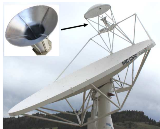
Fig. 1. QRFH (top left) installed on DVA-1, seen just below the sub-reflector.
