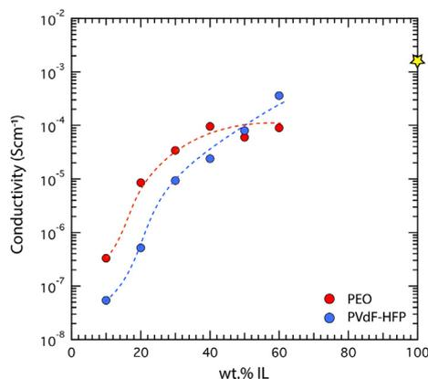
**Fig. 5.** Composition dependence of the ionic conductivity measured at 300 K for membranes based on PEO (red) and PVdF-HFP (blue). The value measured for the neat IL is also shown as a yellow star.
