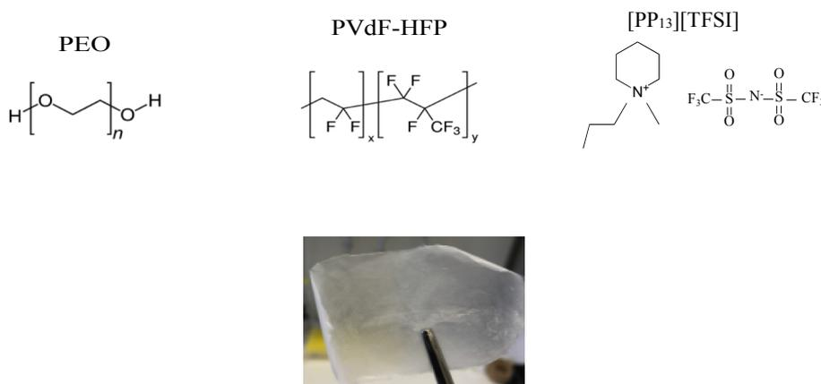
Fig. 1. Molecular structure of PEO, PVdF-HFP, and [PP<sub>13</sub>][TFSI]. A picture of one PEO/IL membrane is also shown.
