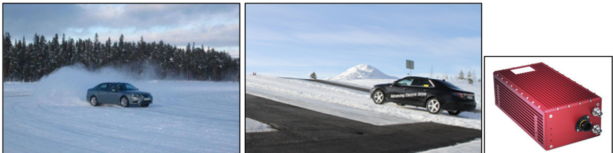
Figure 8 Test vehicles at high side-slip (left) and start at slopes (middle) maneuvers as well as IMU (right)
