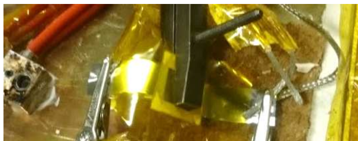
Figure 4.2: The supercapacitor inside a small oven capable of 300°C. The supercapacitor is placed inside a small vise to keep pressure on the electrodes during the measurement.
