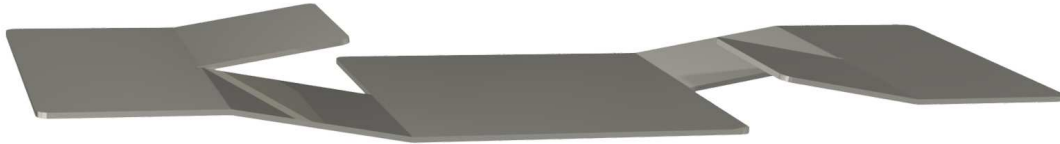
Figure 2.16: A schematic figure showing an electrode that has been shaped to act as a spring during first heating. The electrode has some spring force left even when pushed flat.
