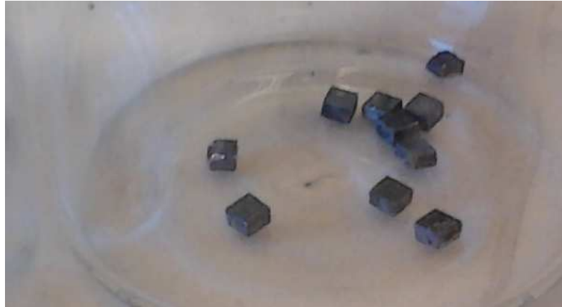
Figure 2.14: The size ( 1.6 \text{ mm} \times 1.6 \text{ mm} \times 1 \text{ mm} ) of the thermoelectric legs in the harvester. The material in this picture is \text{Ba}_8\text{Ga}_{16}\text{Ge}_{30} .
