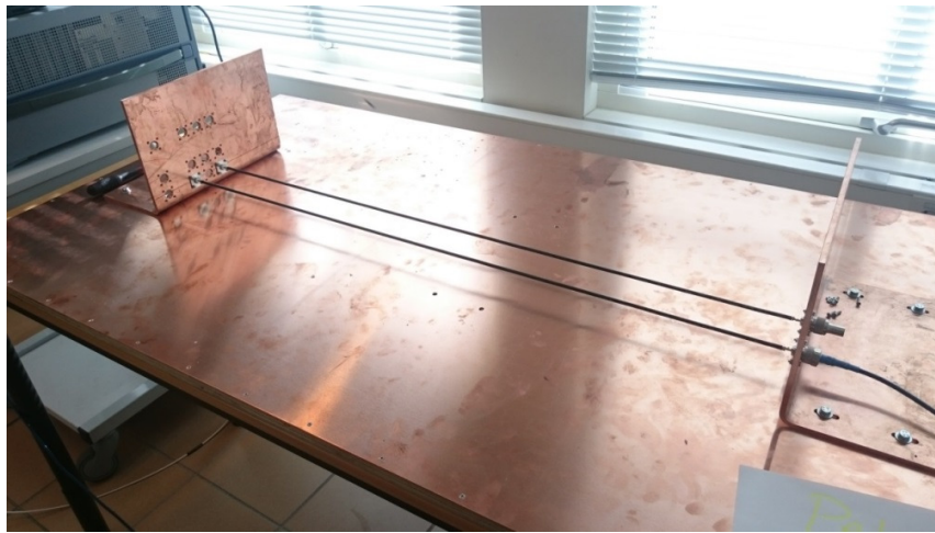
Figure 8.45 - Cable rig for cable measurements over copper plane. Here two RG58 coaxial cables are attached to the N-connectors on the copper plates and additional loads.
