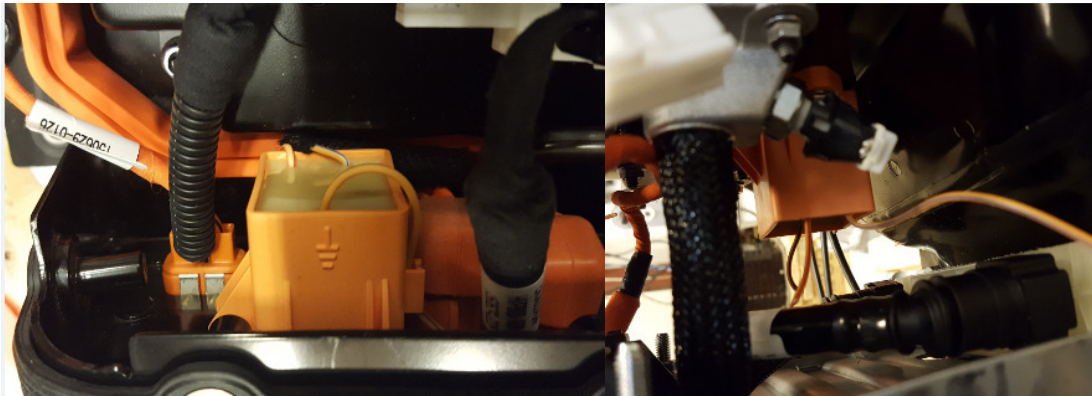
Figure 9.11 - Inert battery pack. The Y-capacitors in each end of the battery. IEM side of the battery to the left and CIDD side to the right
