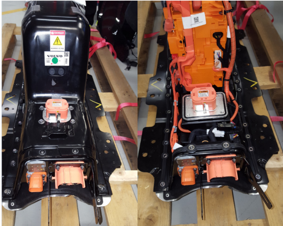
Figure 9.10 - Inert battery pack. The side with the IEM (right) and OBC (left) connector. Here also the MSD (Manual Safety Disconnect) can be seen. With and without lid
