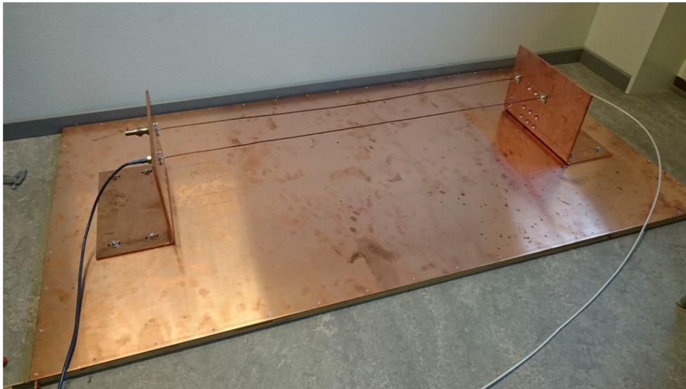
Figure 8.27 Test rig for cable measurements over copper plane. Here two copper cables are attached to the N-connectors on the copper plates and additional loads.
