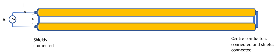
Figure 8.57 - Conceptual drawing showing measurement setup for measurement of differential mode impedance of shielded high voltage DC cable.
