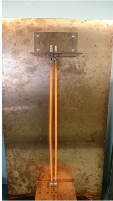
Figure 8.52 - Cable coupling measurement fixture with ground plane
