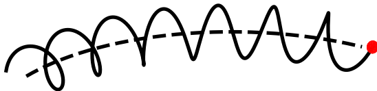
Figure 1.2: Illustration of a particle orbit in a magnetic field. The orbit takes the form of a helix that is wrapped around magnetic field lines, due to the Lorentz force. Often, one is not interested in the gyrating motion around magnetic field lines, and instead studies the guiding-center of the orbit (dashed line).
