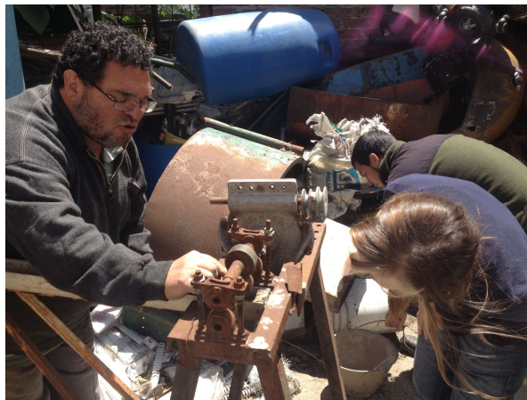
Photo 3: Members of the Cooperativa Reciclando Sueños designed a machine to manufacture plastic ropes reusing old factory machinery
