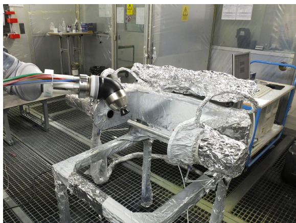
Fig. 3. Measurements of particle size distribution from an Electrostatic Rotary Bell Sprayer using a laser diffraction equipment.
