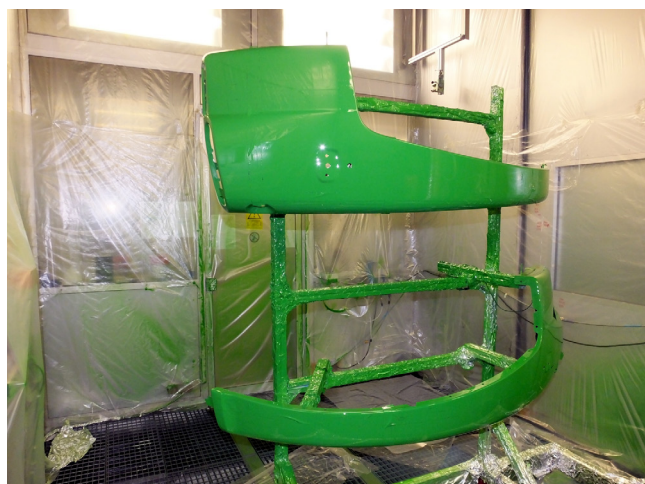
Fig. 7. For validation of the procedure two fenders from the company John Deere were mounted on a rack and painted in the Fraunhofer IPA laboratory.
