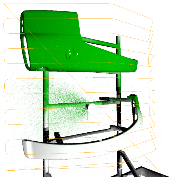
Fig. 9. A snapshot from the painting of the fender in IPS Virtual Paint.
