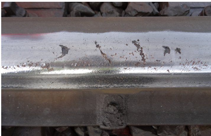
Figure 1.1: RCF cracks and spalls near the gauge corner of a rail.
