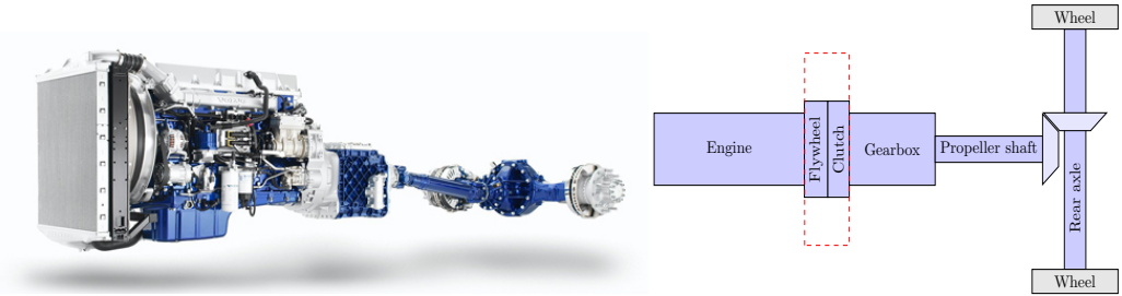
Figure 2.1: Truck powertrain, source: AB Volvo (left) and schematic picture of powertrain (right)
