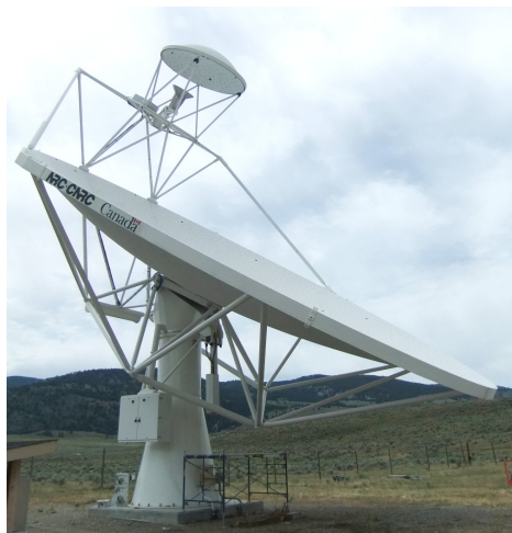
Fig. 3.5: (a) Schematic of the PO+PTD system simulator that models the feed performance on a reflector system; (b) Example of a complete reflector system that can be modeled with the system simulator. The image shows the first SKA Band 1 QRFH prototype mounted on the Dish Verification Antenna 1 (DVA1) in Penticton, BC, Canada in 2016.
