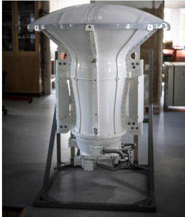
Fig. 3.9: Final prototype of the SKA Band 1 QRFH. Image credit: Chalmers/Johan Bodell.
