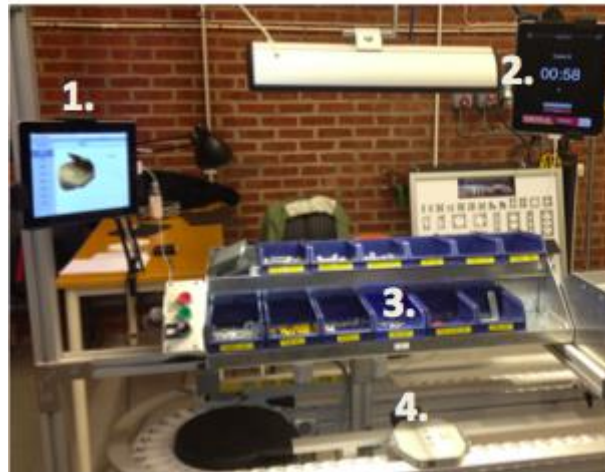
Fig. 3. The experiment area and the experiment set-up. 1. Instructions, 2. Takt time, 3. Material façade, 4. Assembly ground plate
