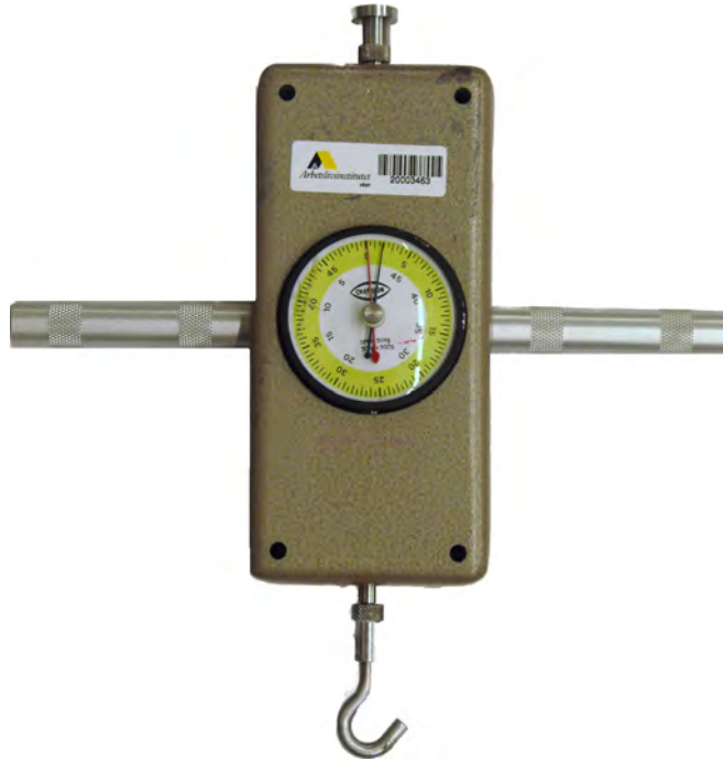
Figure 3.3: Force gauge for measuring push and pull force. The readout is often given in N. Photograph by C. Adams. All rights reserved.
