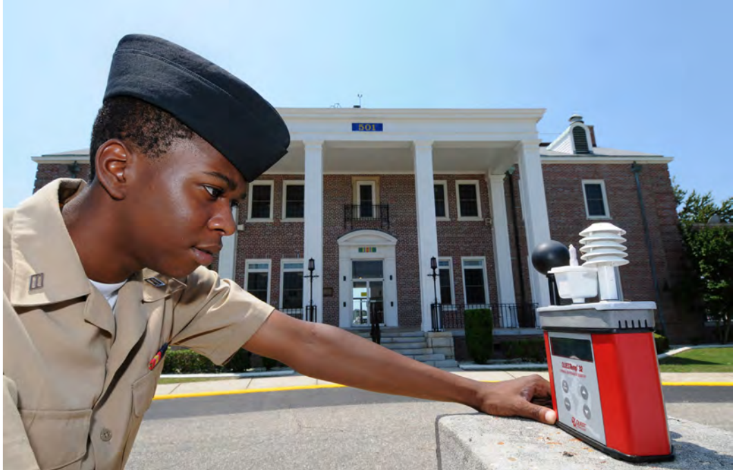
Figure 12.4: Equipment for measuring WBGT being used in the field by a U.S. Navy seaman. U.S. Navy photo by Gary Nichols / Released. The image is in the public domain via www.navy.mil .
