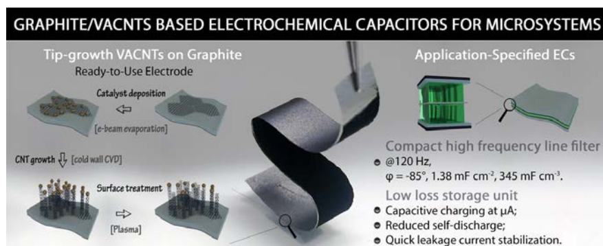
Figure 15. Small size ECs based on graphite/VACNTs electrodes (Paper III).
