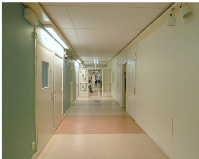
Fig. 8. Portion of a ward in Old hospital showing the corridor-dominated floor layout. The corridor-based design obstructs observation of seating and activity rooms accessed from the corridor. The photo was taken in 2010 after refurbishment for other types of patients. The hospital was subsequently demolished.
