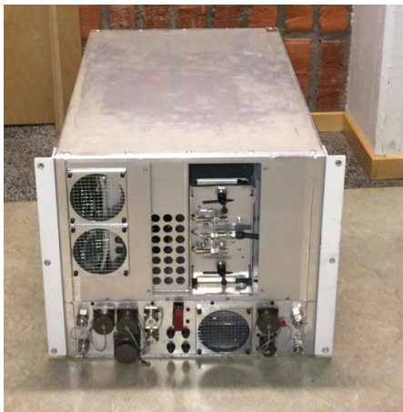
Figure 11. The central part in the measurement system corresponds to a 19" wide sniffer box including a logging computer, a UV fluorescence instrument for SO 2 , a NDIR for CO 2 , and an AIS and GPS receiver and power converter (47 kg, 15 A at 28 V DC).
