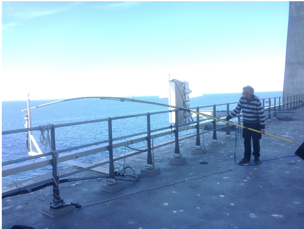
Figure 30. Testing the gas inlet for short time exposure using a premixed \text{SO}_2 and \text{CO}_2 gas corresponding to a 1 % vessel.
