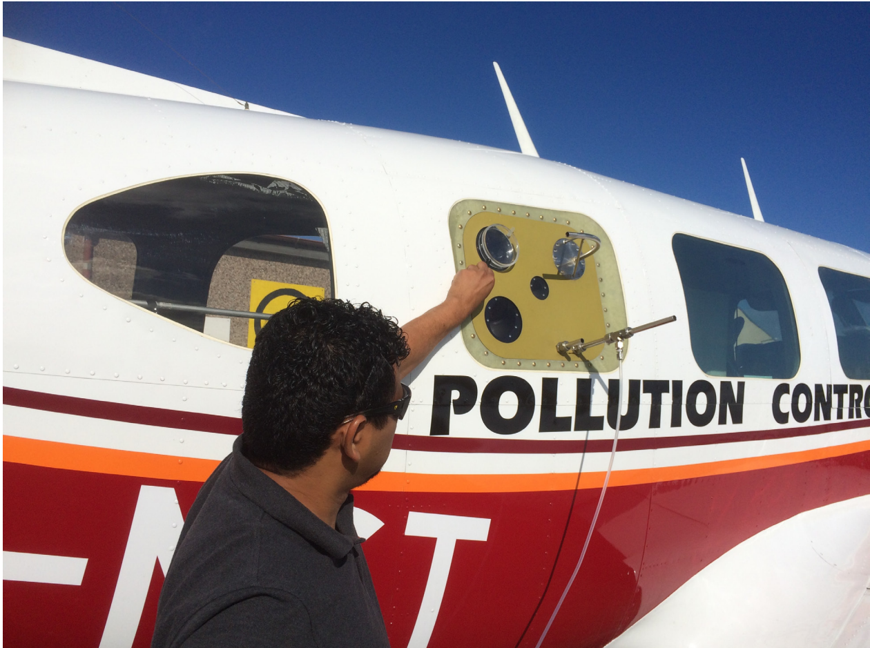
Figure 13. Quality control of the sniffer and optical sensors on the Navajo Piper from Aircraft Aps. The yellow plate includes two windows for optical sensors, a window for a video camera, two inlets for gases and particles, respectively, and one exhaust pipe. The optical system is checked by holding gas cells filled with known concentrations of SO 2 and NO 2 in front of the telescopes. The sniffer system is calibrated by flushing premixed calibration gas in front of the gas inlet using a Teflon tubing.
