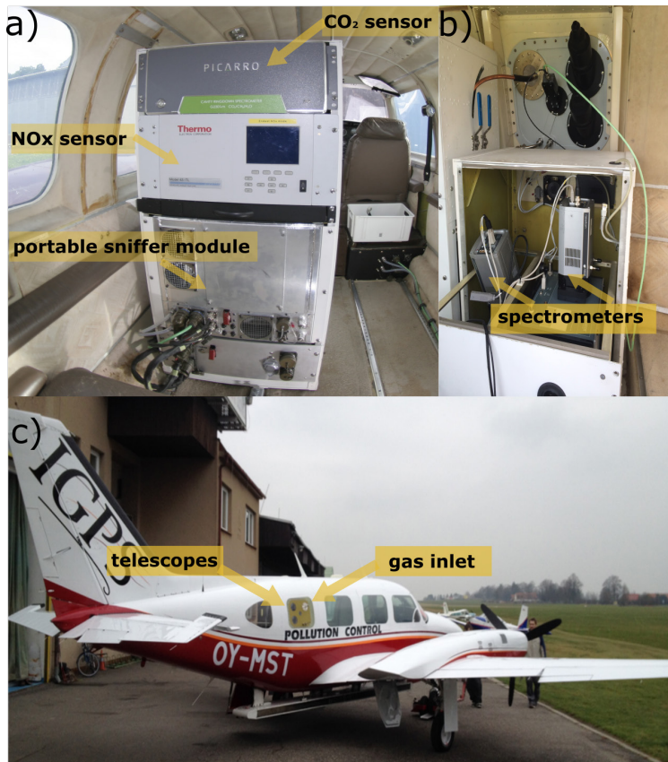
Figure 10. Airborne measurements system: (a) Sniffer installation in the airplane cabin, (b) Spectrometers installed in the airplane cabin with their corresponding telescopes on the upper side, (c) Metallic structure holding the telescopes of the optical system and the gas inlet.
