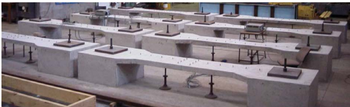
Figure 4.11 Geometry and dimensions of the restrained slab specimens and general view of the slabs in during the testing period, from Nejadi and Gilbert [42].
