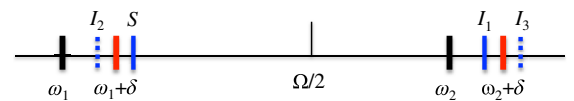
FIG. 6. Four-mode structure of the amplified output field for the detuned signal. Black indicates the cavity resonances, while red marks the parametrically coupled strong-field modes (for \Delta_S = 0 ); the solid blue lines indicate the signal ( S ) and the primary idler ( I_1 ) with the frequencies \omega_1 + \delta + \Delta and \omega_2 + \delta - \Delta ; the dashed blue lines indicate secondary idlers ( I_{2,3} ) with the frequencies \omega_1 + \delta - \Delta and \omega_2 + \delta + \Delta .
