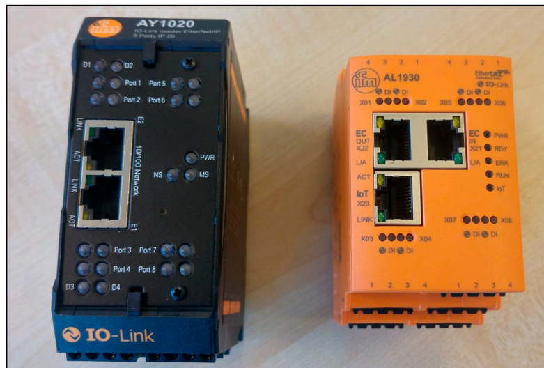
Figure 6. On the left: IO-Link gateway used for the described application (ifm AY1020). On the right: Internet of Things (IoT)-enabled IO-Link gateway (ifm AL1930).
