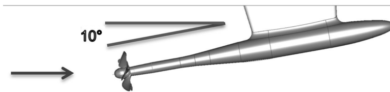
Figure 6.20: Inclined propeller towards the incoming flow in experiment setup
