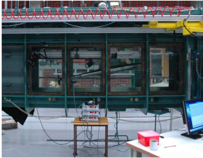
Figure 6.19: Experimental setting of the propeller cavitation tests
