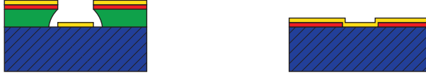
Figure 4.2: (left) With the presence of the undercut, the metal layer (yellow) is not continuous and allows the remover to access the resist. (right) Without the undercut and lift-off layer, the metal forms a continuous layer on top and remover can't access the resist.
