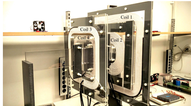
Fig. 1. Photo of the air-wound coils used in the WPT system prototype with four magnetically coupled resonators.
