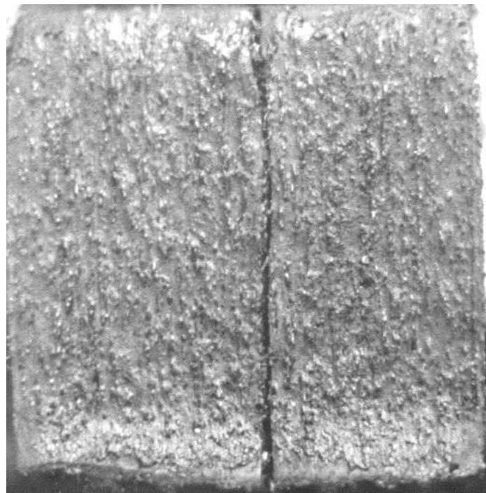
Figure 7.6 Characteristic surface structure for material B. Environment temperature 25 °C. Sliding speed 0.27 m/s. Pressure 0.847 MPa. Sample size 10 mm · 10 mm.
