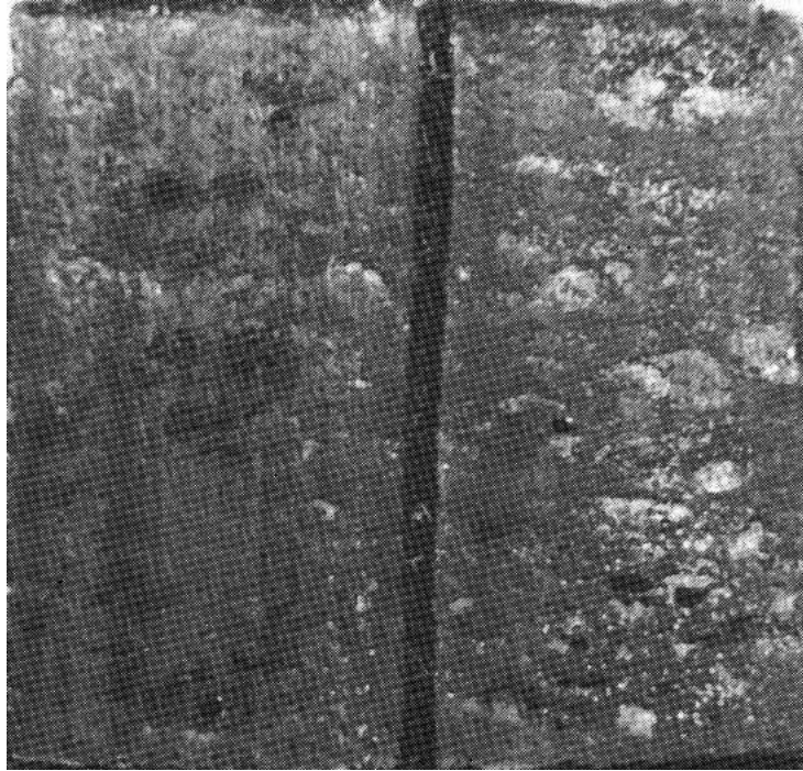
Figure 7.1 Characteristic surface structure for material A. Environment temperature 25 °C. Sliding speed 0.27 m/s. Pressure 0.136 MPa. Sample size 10 mm · 10 mm.
