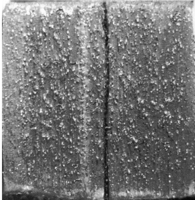
Figure 7.5 Characteristic surface structure for material B. Environment temperature 25 °C. Sliding speed 0.27 m/s. Pressure 0.491 MPa. Sample size 10 mm · 10 mm.
