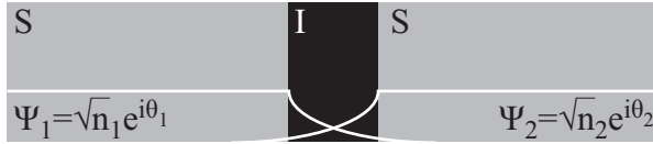
Figure 2.2: A superconductor-insulator-superconductor (SIS) junction. The white line indicates the BCS wavefunction, and the fact that the wavefunctions \Psi_1 and \Psi_2 overlap indicate that Cooper pairs can tunnel.
