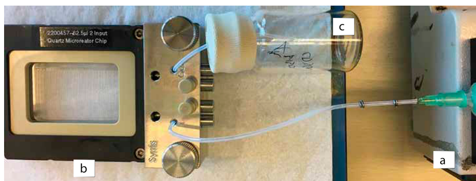
Figure 4. Picture of the chip-based microreactor setup. (a) Syringe pump for injecting the solutions into the microfluidic chamber. (b) Quartz microreactor (62.5 \mu\text{L} ) in which the PPG-protected esters are irradiated with a 254 nm UV lamp. (c) Collection vial that contains the reagents for the CuAAC reaction.
