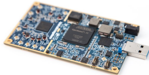
Figure 1: The LimeSDR front-end, which has been chosen for this project, is based on field programmable RF transceiver technology, combined with FPGA and microcontroller chipsets.
