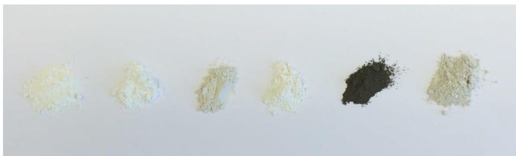
Figure 31 From left to right: virgin rutile pigment, virgin dolomite extender, virgin mica extender, mix of virgin pigments corresponding to the one in the pyrolysis ash, ground pyrolysis ash, heat treated pyrolysis ash.
