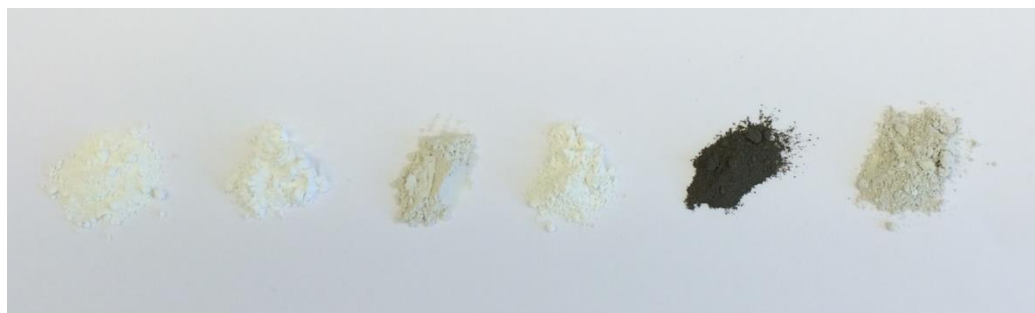
Figure 4 From left to right. Virgin rutile pigment, virgin dolomite extender, virgin Mica extender, mix of virgin pigments corresponding to the one in the pyrolysis ash, grinded pyrolysis ash, heat treated pyrolysis ash.
