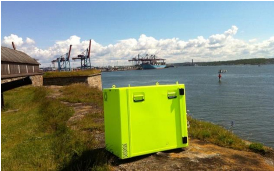
Figure 1. The yellow box developed for automatic emission measurements.
