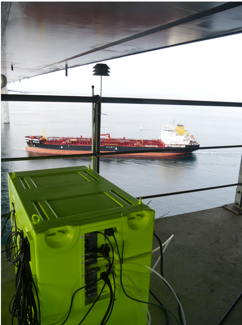
Figure 9. Fixed sniffer system installed at the Öresund Bridge between Sweden and Denmark. The gas is extracted from the funnel shaped gas inlet which is connected to the railing.
