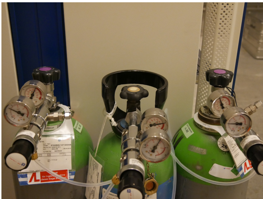
Figure 5. Premixed calibration gases of CO 2 , SO 2 and NO x are connected to the sniffer system via electrically controlled gas valves.
