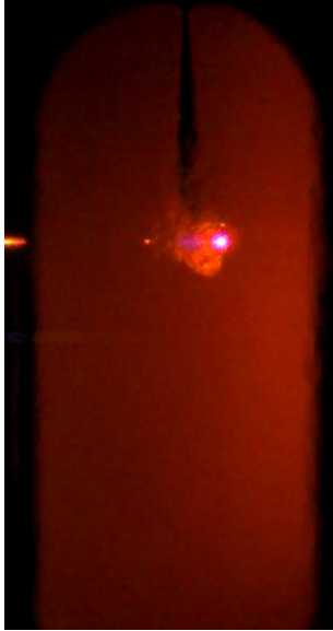
Figure 4: Laser ignition test with pure ethanol
