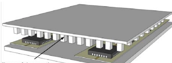
Figure 4. Tx and Rx MMIC amplifier chains packaged by lid of nails. The configuration has also been built and measured.
