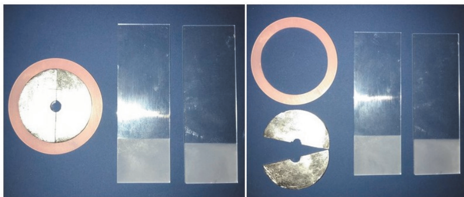
Figure 10. Split stainless steel mold
