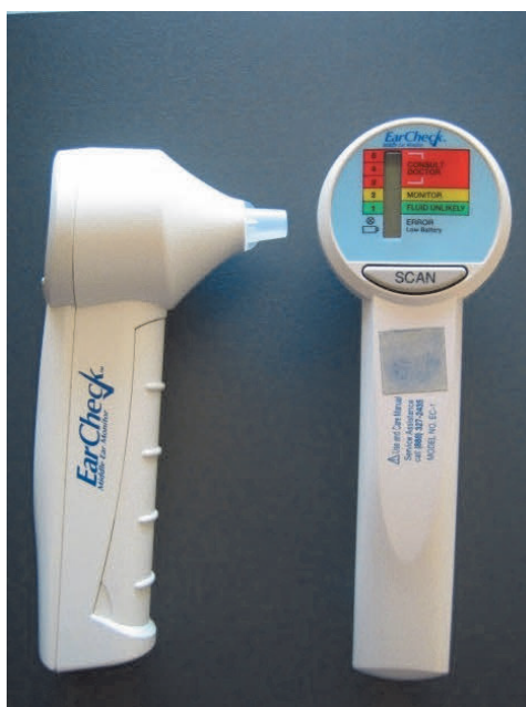
Figure 9. Consumer model of a spectral gradient acoustic reflectometer (EarCheck™ Middle Ear Monitor).
