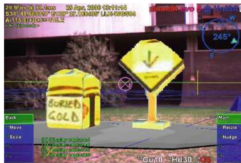
Figure 5: Indoor user has added a signpost to help outdoor user to navigate [29].
