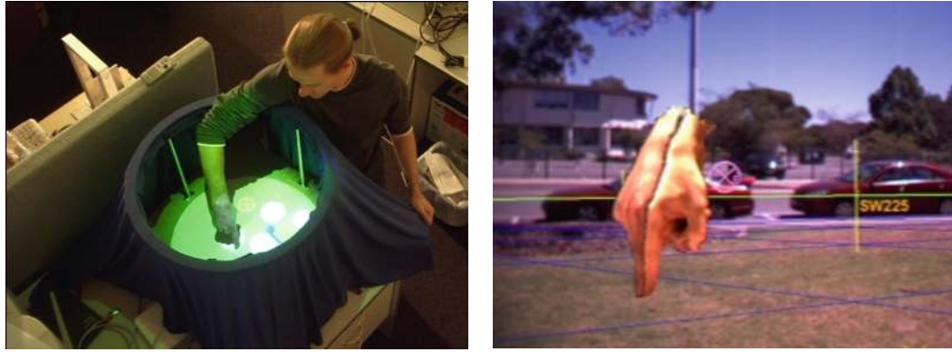
(a) Indoor specialist using interface of the Hand of God system. (b) View for outdoor specialist with virtual hand of indoor specialist.
