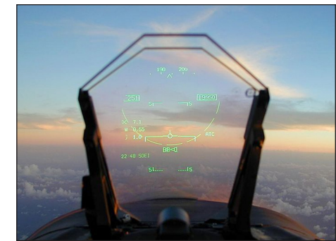
Image 2. Head-up display in an aircraft.
