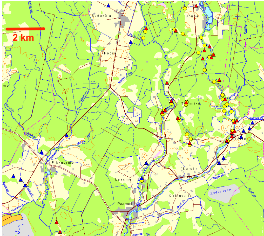
Figure 4. Lime production facilities in Kursi parish identified by the end of 2009. Red triangles – preserved limekilns or remains; Blue triangles – limekilns mentioned in written sources but indistinguishable on the landscape; Yellow circles – limestone quarries (Tvauri & Saimre 2010, fig. 1.)
