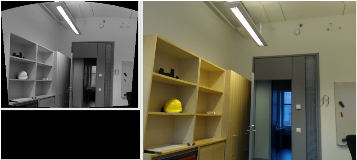
Figure 6.5: Functionality of the warper: the original image on the right, and the resized, grayscale warped image on the left. The image is warped to represent the change when the camera is rotated 10 degrees on the y-axis.
