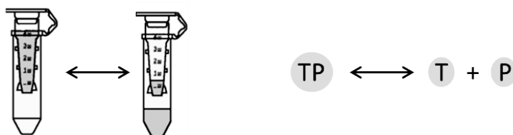
Figure 19. The ultrafiltration technique is based on the equilibrium between the protein bound and unbound tannin during repetitive centrifugation with the filter unit. T: tannin, P: protein.
