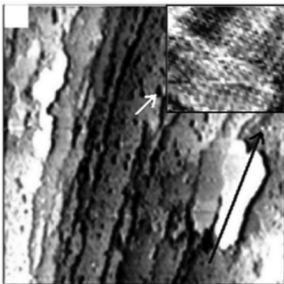
Figure 25. STM image of an InN island. The scale is 800 nm × 800 nm. The inset shows a zoomed in image taken from the top of a separate island.
