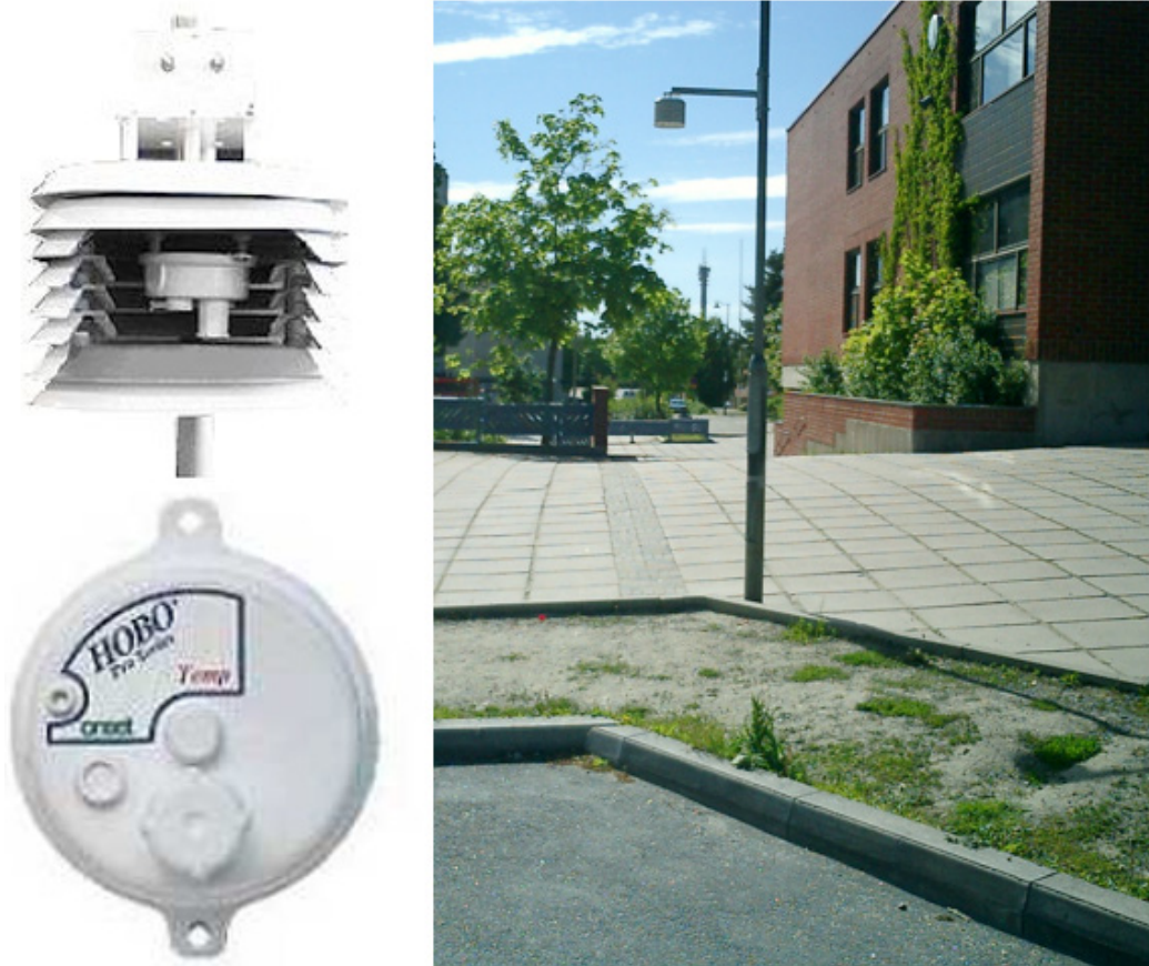
Figure 6. Hobo H8 Pro temperature loggers. Loggers are placed inside radiation shields on poles at 3 m elevation above the immediate surrounding ground. The site on the photo is in the Varissuo suburb (Figure 7, logger site no. 54).
