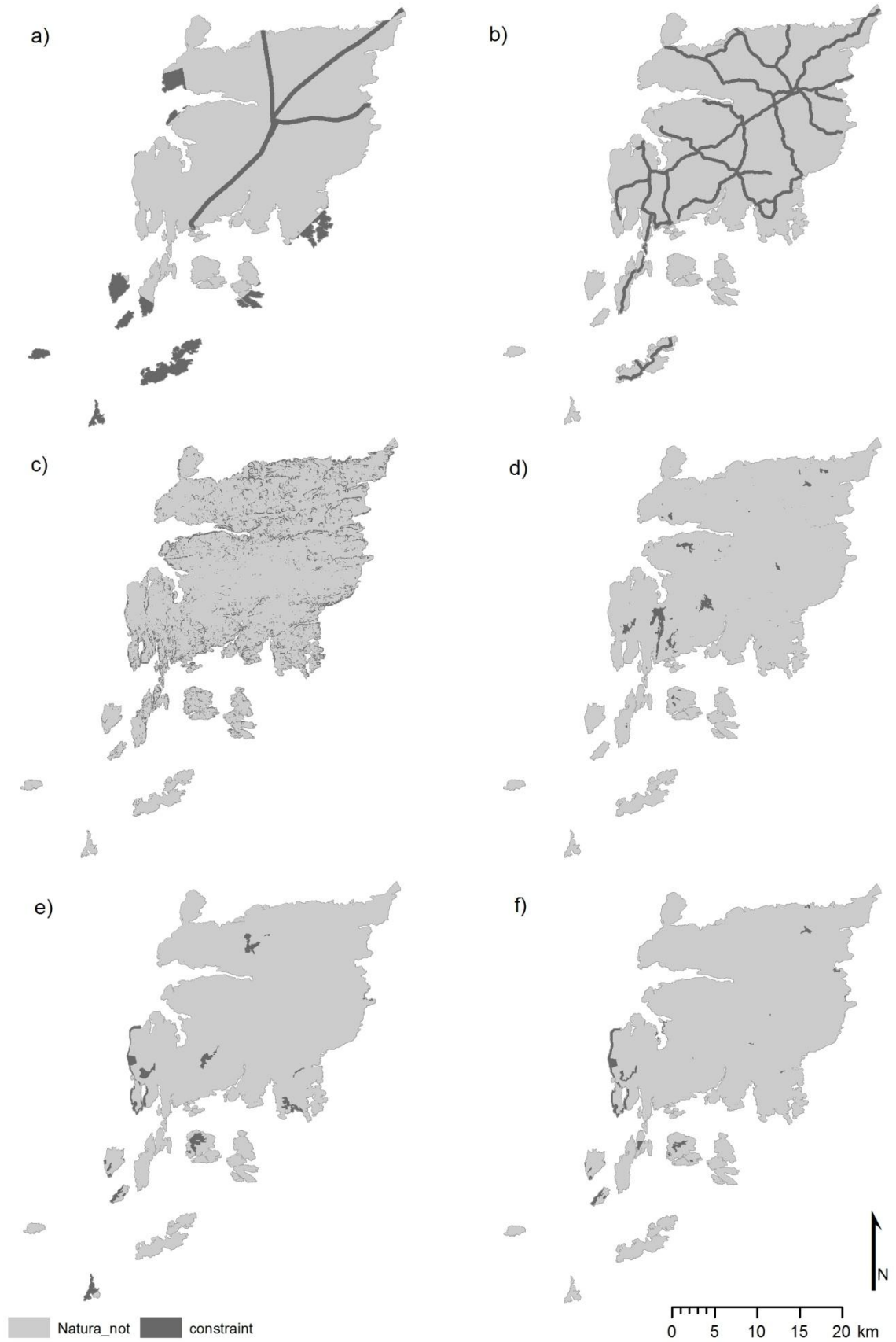
Constraints. a) Grid, b) state roads, c) steepness, d) lakes, e) Natura 2000 areas and f) protection areas.
