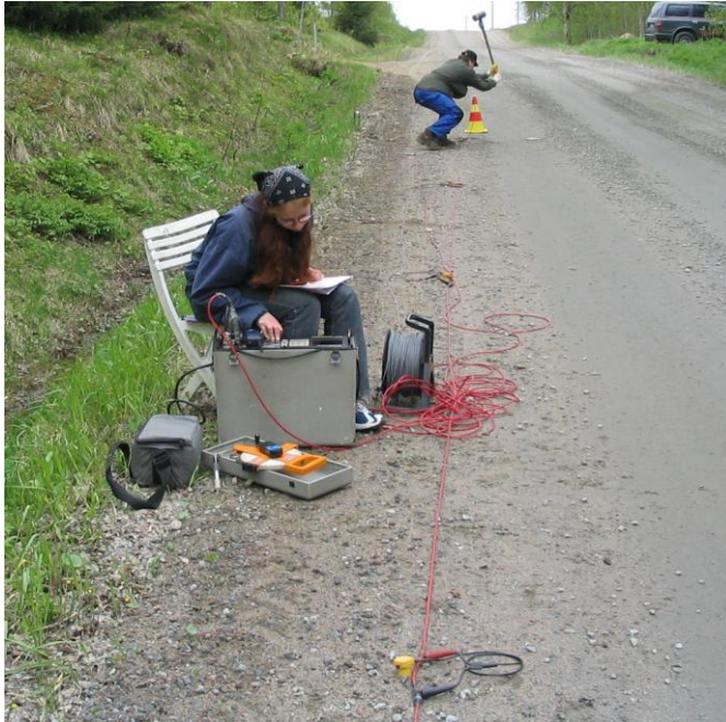
Fig. 116. Refraction seismic sounding next to the Höytiä test well no. 892015 in the municipality of Uurainen, Central Finland, in the summer of 2004. Photo adopted from Lindsberg (2011). Original photo Ossi Alho/CETECF.
