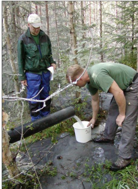
Fig. 31. Yield determination during air-flushing of the Ristimäki test well no. 077081 in the municipality of Hankasalmi, Central Finland, in August of 2005. Drilled well depth at the moment the photo was taken was 61 m and Q \sim 2,500 \text{ Lhr}^{-1} ; the final well depth was 91 m and Q = 9,000 \text{ Lhr}^{-1} . Photo Kari Illmer/CETECF.
