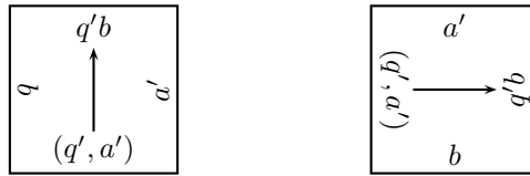
(a) The tile for read-write operation \delta(q, a) = (q', a', \triangleleft) . (b) The tile for read-write operation \delta(q, a) = (q', a', \triangleright) .
