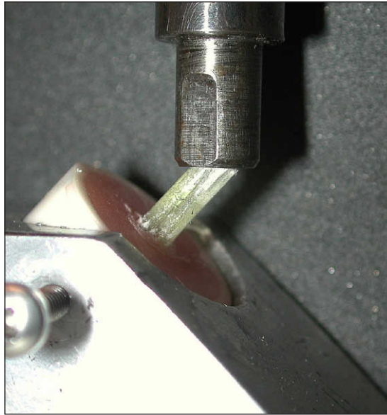
Figure 12. Cantilever bending test of the specimen.
