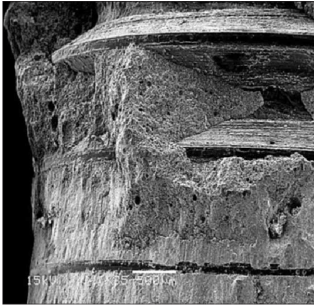
Figure 16. SEM micrograph of fracture surface of polymeric-threaded FRC device after push-out test. Fracture occurred through outer layer of FRC threads, suggesting that main failure reason was low cohesive shear strength of plaster.
