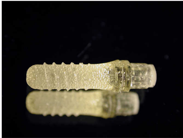
Figure 2. One-piece design of threaded FRC implant.
