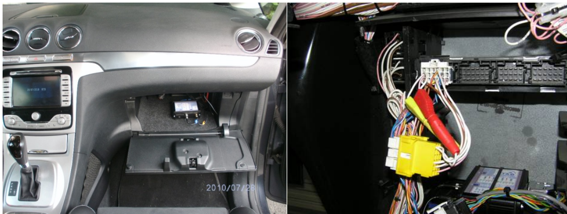
Figure 10: German-1 VMC - Placement of DAS inside glove compartment (Ford) and inside truck cabin (MAN).
