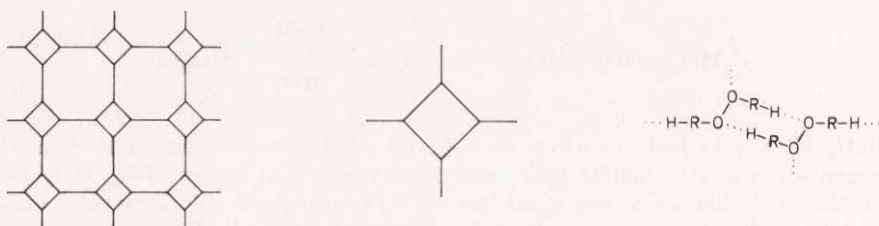
Fig. 9. The idealized structure of the anion in \gamma\text{-BaO}_2 \cdot 2\text{H} \cdot \text{O} (Alternative I).
