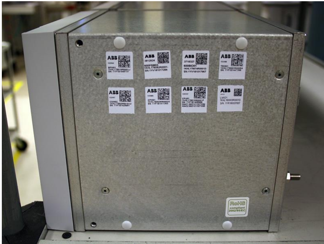
Picture 16. A relay case and module labels
