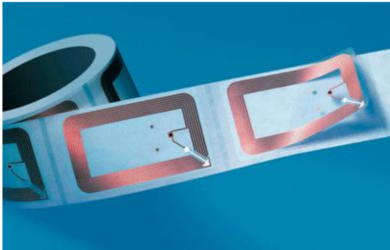
Picture 5. Passive RFID tags on a roll. (Libramation)
