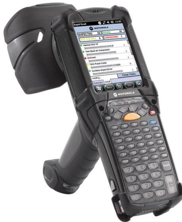
Picture 7. An example of a handheld RFID reader (Motorolasolutions)
