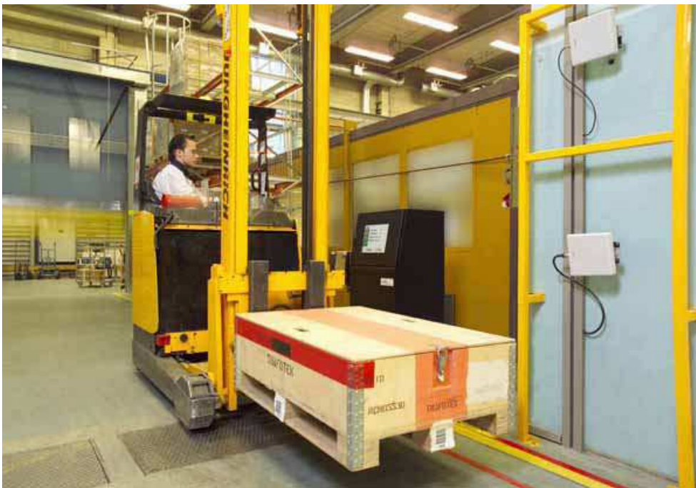
Figure 15 RFID Forklift Drive-Through Gate and a Pallet with RFID Tag at ABB Drives (ABB Inc. Press Release, RFID Lab Finland ry 2005: 2)
